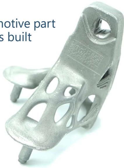
automotive part after 200.000 km wear out test
