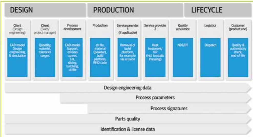
Picture 3: The process chain for 3D printing.
